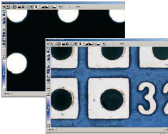
The lighting panel offers software control for surface illumination, back lighting and also TTL lighting, if available. The surface illumination tool allows directional control of the lighting as well as for intensity, which is fully automatic under CNC playback.
